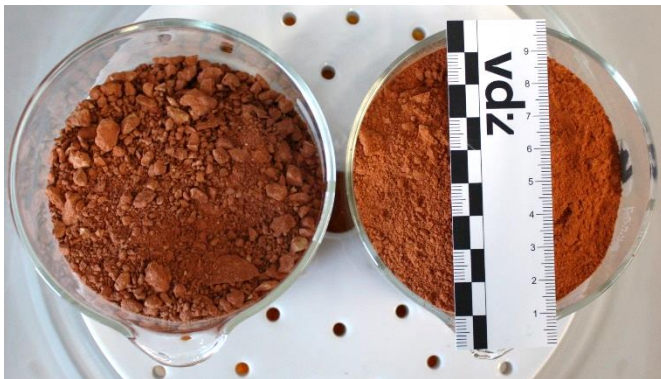
Figure 1 Sample for storage experiments. left: crushed coarse calcined clay (g); right: finely ground sample (f)
